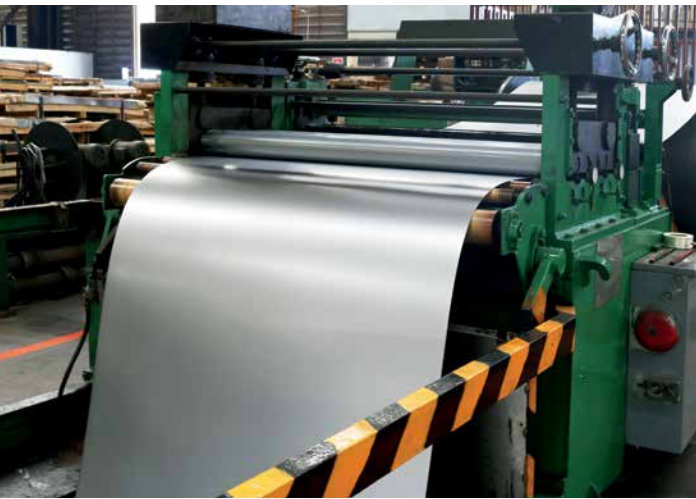
Figure 18. Such rolled steel is modified to client specifications by Pacesetter’s Service Center.
