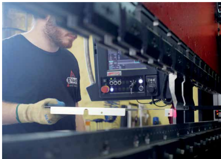
Joey Klein uses a brake press to bend parts for a generator at Evans Tool & Die/Evans Metal Stamping, Inc. Photograph from Evans Tool & Die/Evans Metal Stamping, Inc.
