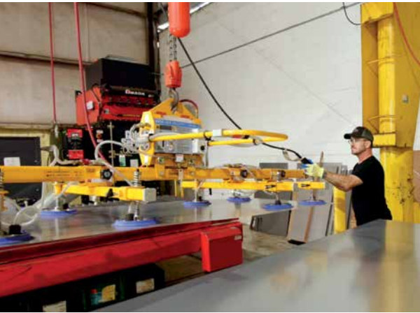
Figure 14. At Evans Tool & Die/ Evans Metal Stamping, Inc., Kevin Klein loads sheet metal into a fiber laser cutting machine to fashion a part for the firearms industry. Photograph from Evans Tool & Die/ Evans Metal Stamping, Inc.
